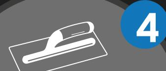
Once your trowel is loaded, Apply product to the surface swiping from bottom to top. Aim to keep the application approximately 3-4mm thick for the best coverage.
